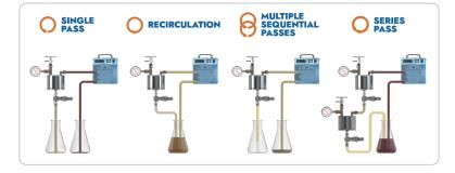
For a single pass usage, we suggest to run at very low flow rate compared to recirculation process, which can be run at higher flow rate. Click on the picture below to access the video on E-PAK purification methods.
